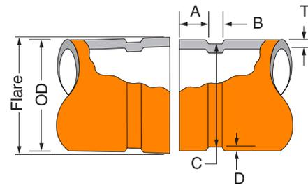
End Guard (EG) roll groove is designed for standard or heavier wall thickness pipe to be joined by Fig. 7004 with EG® gasket couplings.
