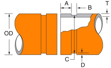
End Guard (EG) cut groove is designed for standard or heavier wall thickness pipe to be joined by Fig. 7004 with EG® gasket couplings. Gruvlok EG fittings are grooved in accordance with these dimensions.
