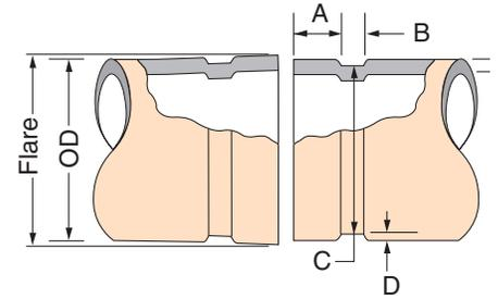
**COLUMN 1** – Nominal tubing size ASTM B88
